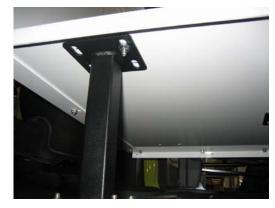
Attach assembly to K9 floor using ¼" x ¾" carriage bolts and serrated nuts
